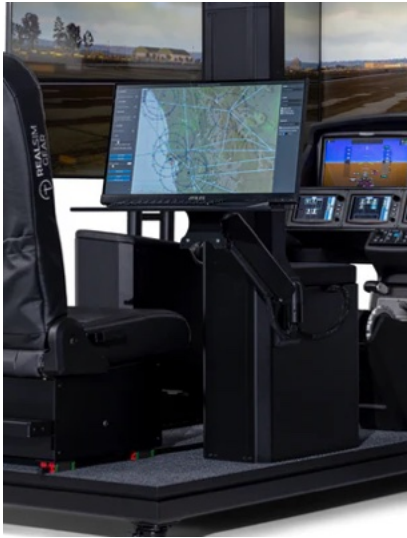
Image 14. Instructor station showing moving map, vector airways and current airplane position.
