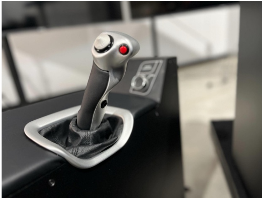
Image 9. Control yoke/stick showing yoke mounted switches.
