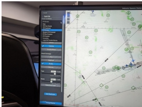
Image 15. Instructor station displaying weather controls and systems malfunction controls interface.
