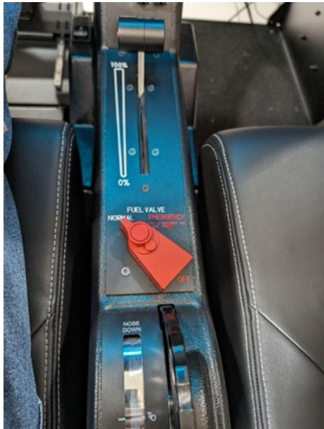
Image 11. Engine control lever, flap selector - mixture,fuel pump and selectors
