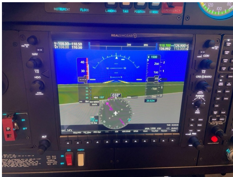
Image 8. Co-Pilot side of instrument panel showing full screen MFD
