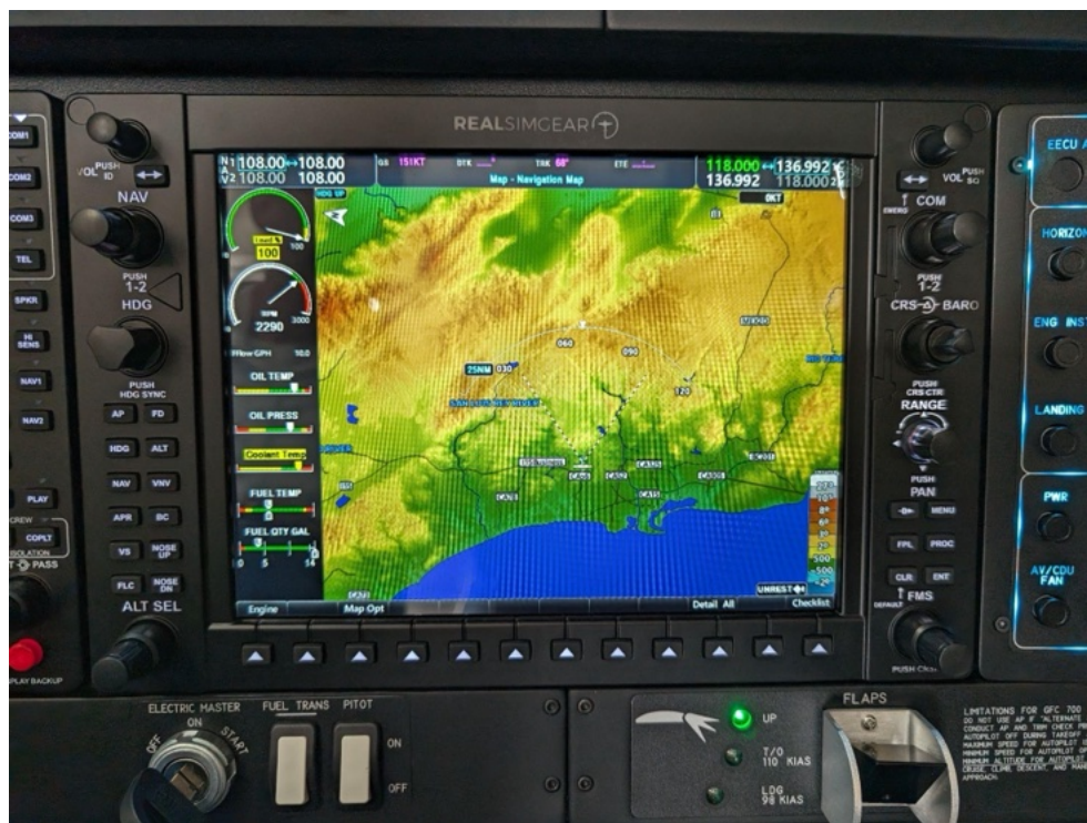
Image 8. Co-Pilot side of instrument panel showing full screen MFD
