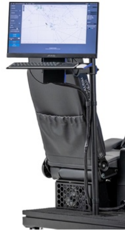
Image 15. Instructor station showing moving map, vector airways and current airplane position.
