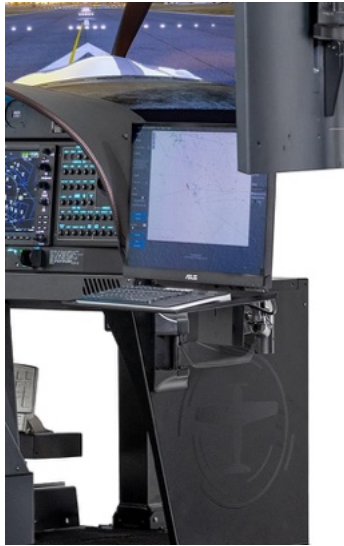
Image 15. Instructor station showing moving map, vector airways and current airplane position.
