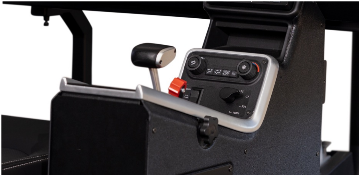
Image 11. Engine control lever, flap selector - mixture, fuel pump and selectors
