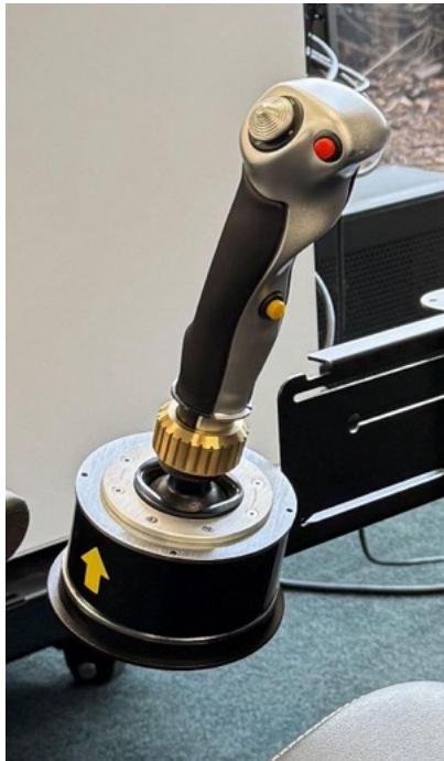
Image 9. Control yoke/stick showing yoke mounted switches.
