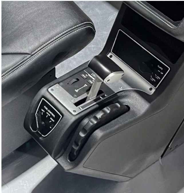
Image 11. Engine control lever, flap selector - mixture, fuel pump and selectors
